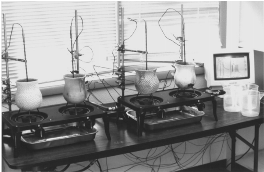
Fig. 5. Arrangement of vessels and temperature probes during cooking effectiveness and use-life experiments.
